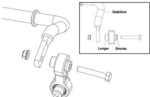
3. Install the lower end of ①Stabilizer end link onto the lower control arms and tighten using the original bolts and nuts.
