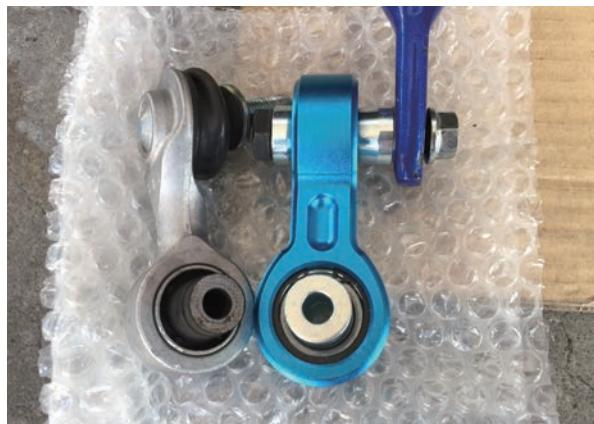
2. Locate the upper end of the end-link to the stabilizer and tighten using provided ②Bolts and ③Nuts. Notice that the side with pivot longer should be installed to the stabilizer. (See figure 1&2)
